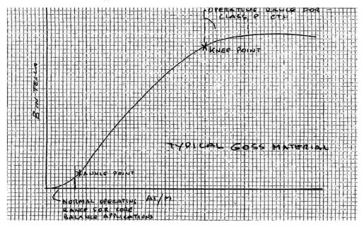
As you can see the performance specified is at 10 or 20 times rated current, this does not ensure that the Current Transformer will generate sufficient output to operate a typical core balance protection primary sensitivity of typical 250mA or 500mA. This is due to the fact that typical GOSS material has magnetizing characteristics that are not linear but in fact rise up slowly to what is termed the ankle point of the curve.
